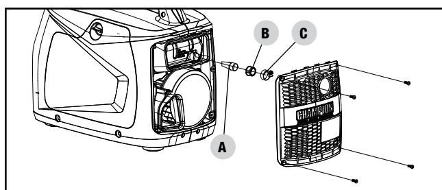
4. Remove the spark arrestor screen.
