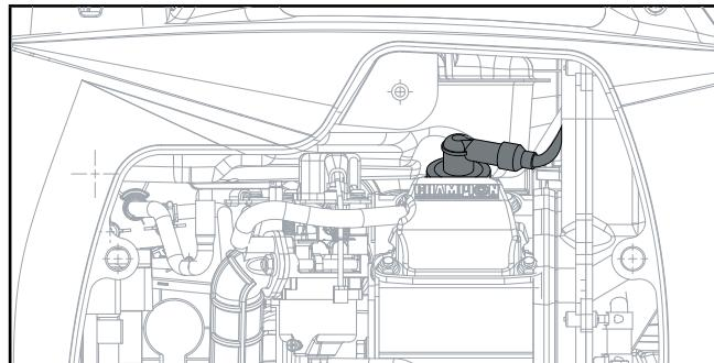
2. Remove the spark plug wire from the spark plug.
